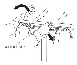
Figure 15. Adjusting Direction of Lighting Units Turning Lights Individually
